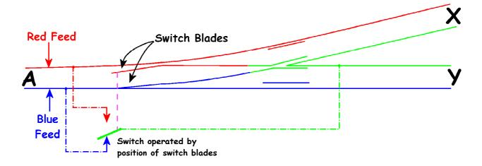
The point is set for traffic to pass between A and X.
