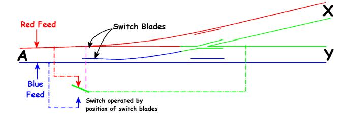
The point is set for traffic to pass between  $\boldsymbol{A}$  and  $\boldsymbol{Y}$ .
